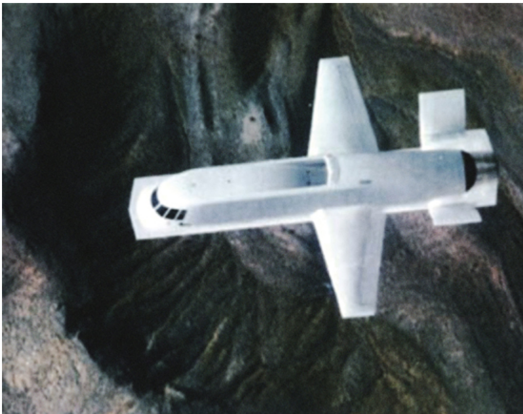
Nicknamed “the Whale,” Northrop’s TACIT BLUE was an early stealth technology demonstrator. It first flew at Groom Lake in 1982 and was retired in 1985. The Air Force made the existence of the black aircraft public in 1996. Both images: USAF
